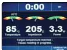
The large color screen on the RFG PLUS displays real-time temperature, impedance and power values
